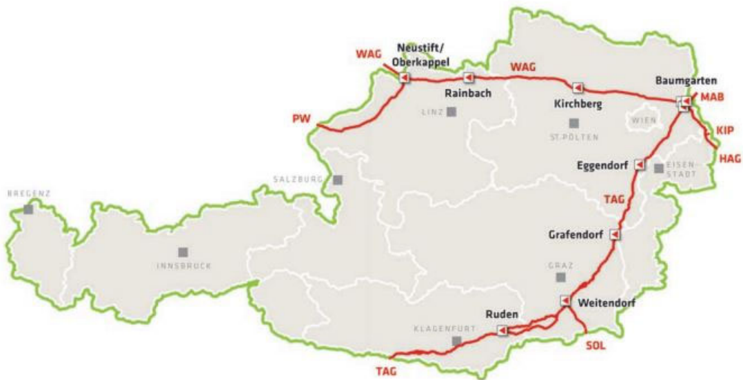
Figure 43: Main Austrian international pipelines
