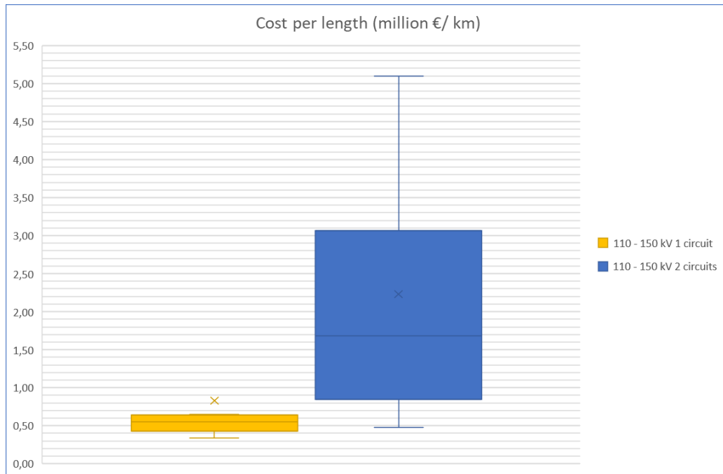
Figure 5. UIC indicators for underground cables of 110-150 kV voltage range with 1 and 2 installed circuits; million EUR/km
